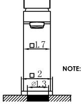
NOTE: Faucet Is Designed To Be Installed Through A 1" Hole (1-1/2" Max. Diameter)
