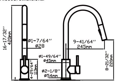
NOTE: Faucet Is Designed To Be Installed Through 1" Hole (1-1/2" Max. Diameter)
